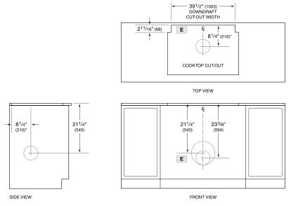
$^{\star}6^{\prime\prime}$  (152) back from countertop cut-out when internal blower is rear mounted.
