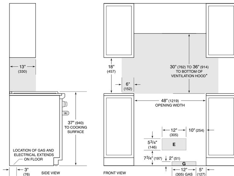
*\*Without ventilation hood, 42" (1067) minimum clearance countertop to combustible materials, charbroiler and GR488 require non-combustible materials. NOTE: Shaded area above countertop indicates minimum clearance to combustible surfaces, combustible materials cannot be located within this area. For island installation, 12" (305) minimum clearance back of range to combustible rear wall above countertop.*
