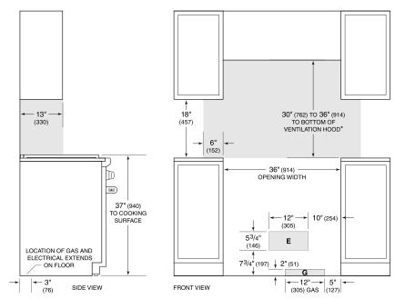
\*Without ventilation hood, 42" (1067) minimum clearance countertop to combustible materials, charbroiler requires non-combustible materials. NOTE: Shaded area above countertop indicates minimum clearance to combustible surfaces, combustible materials cannot be located within this area.
