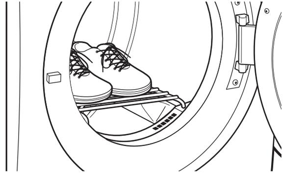
3. Place wet items on top of the drying rack. Allow space around items for air to circulate. The drying rack does not move, but the drum will rotate; be sure to leave adequate clearance between items and the inside of the dryer drum. Make sure items do not hang over the edges or between drying rack grille.
