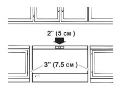
Allow at least 3 in. (7.5 cm) of air space on both sides of the freezer and 2 in. (5 cm) between the back of the freezer and the wall. Leave room above the freezer to open the lid.
