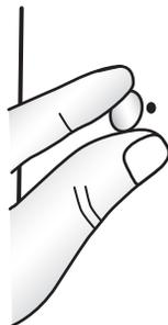
10. Remove door hinge hole plug from the refrigerator door. Move to opposite side.
