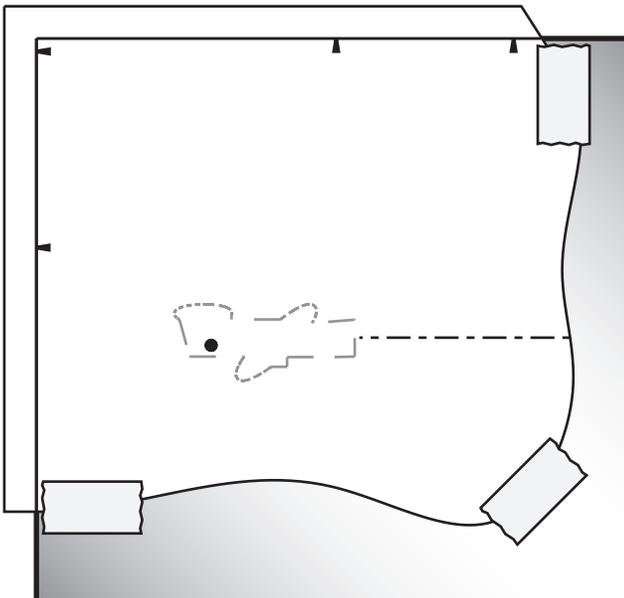
5. Using the cutout as a guide, press the brand badge onto the freezer door making sure that the hole is completely covered.
