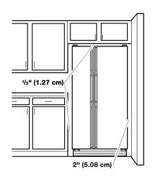
IMPORTANT: This refrigerator is designed for indoor household use only. To ensure proper ventilation for your refrigerator, allow for a  $\frac{1}{2}$ " (1.27 cm) space on each side and at the top. Allow for 1" (2.54 cm) of space behind the refrigerator. If your refrigerator has an ice maker, make sure you leave some extra space at the
