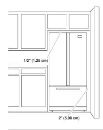
To ensure proper ventilation for your refrigerator, allow for a 1/2" (1.25 cm) of space on each side and at the top. Allow for a 1" (2.54 cm) space behind the refrigerator. If your refrigerator has an ice maker, allow extra space at the back for the water line connections. When installing your refrigerator next to a xed wall, leave a 2" (5.08 cm) minimum space between the refrigerator and wall to allow the door to swing open.
