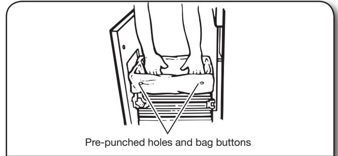
**NOTE:** The ram can and will tear improperly installed bags.
