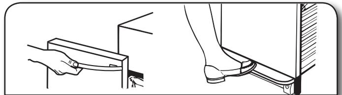
**NOTE:** Pressing the foot pedal opens the drawer only 3" to 6" (7.6 cm to 15.2 cm), dependent upon the load.
