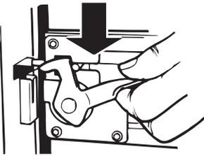
Remove the drawer side by lifting it out of the drawer.
