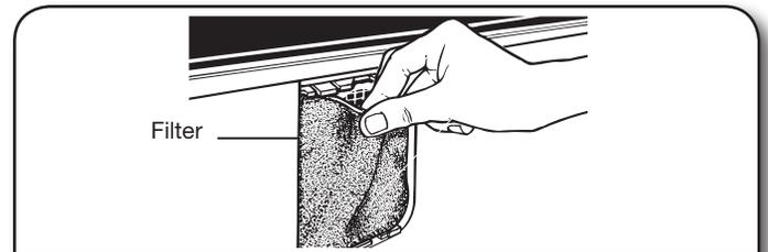
3. To replace air filter, push the replacement filter into place.
