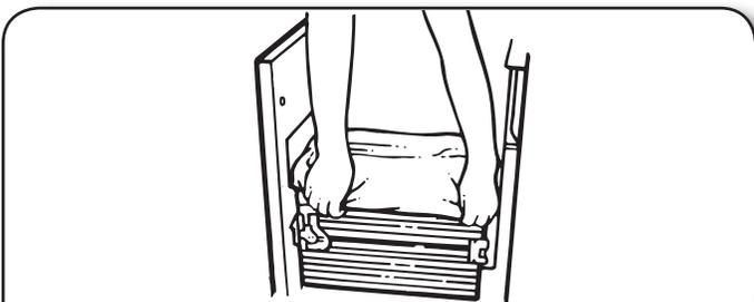
2. Lock bag in place by pulling the four pre-punched holes over the bag retainer buttons. Holes will expand over the buttons without damaging the bag.
