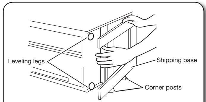
**NOTE:** Before returning the compactor to the upright position, adjust the height of the compactor as necessary using the following "Height Adjustment" instructions.
