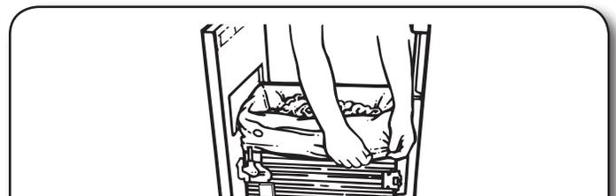
3. Release drawer side latch. Tilt drawer to the right. This releases pressure on the bag making it easier to remove the bag.
