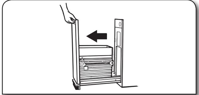
**NOTE:** Look to see how the drawer rollers move in the tracks and disengage. It will be easier to replace the drawer after you have finished cleaning.
