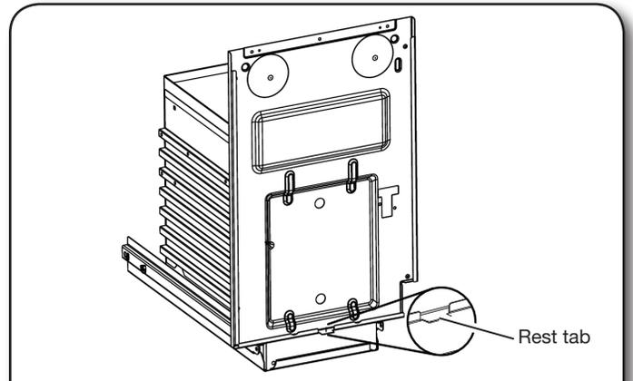
Secure the custom panel to the exterior drawer front by using four #8 x 1" wood screws from the inside drawer front. There are seven holes available for use.
