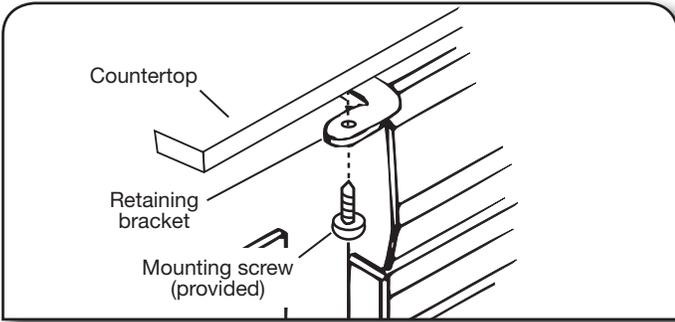
**NOTE:** If the retaining brackets cannot be attached to the underside of countertop, see the “Cabinet-face Mounting” section.
