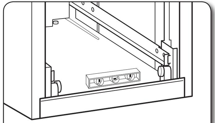
7. Using the two #8-18 x 1/2" (13 mm) screws (provided), fasten the retaining brackets to the countertop with the mounting screws.
