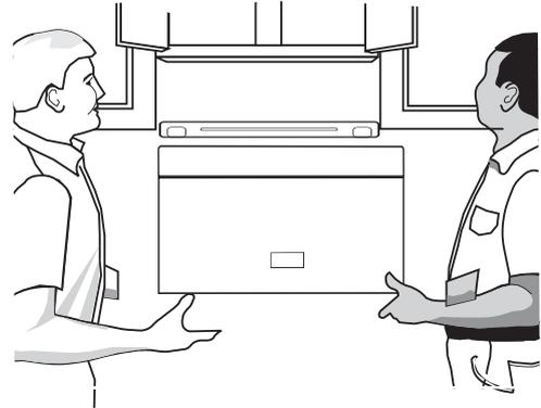
1. Lift microwave, tilt it forward and hook slots at back bottom edge onto four lower tabs of mounting plate.
