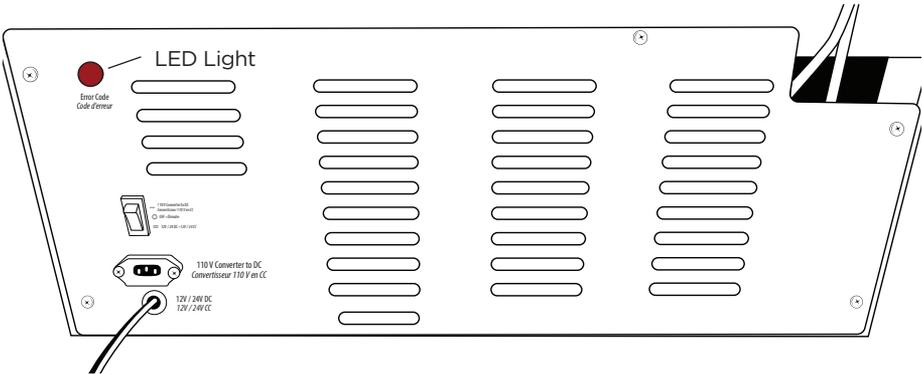
**Remove screws from back plate to access the 15A in-line fuse, water catch basin, and compressor compartment**
