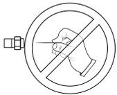
**WARNING - DO NOT** use a pin or wire when cleaning the burner orifice as damage can occur to the precision opening. This can cause damage to the refrigerator or create a fire hazard. It will also create **extremely dangerous** levels of carbon monoxide.
