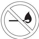
**WARNING -** The gas button **D (Fig. #5)** must be manually depressed to allow gas pressure to flow to the burner orifice. Be sure to apply the leak check solution before depressing the safety shut-off. **DO NOT** allow any open flame, sparks, smoking, etc. in the area of the test. **DO NOT** depress safety shut-off for over 30 seconds.
