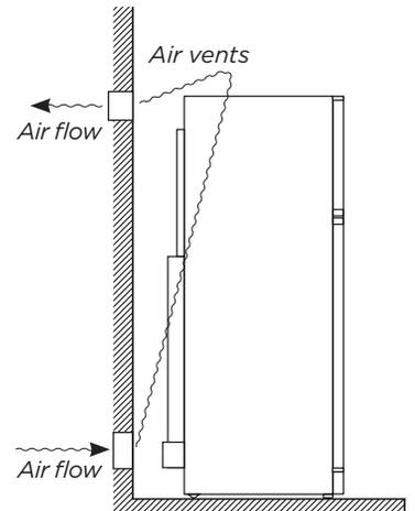
Fig. 4 Air flow - to release heat trap
