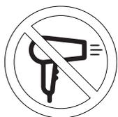
**DO NOT USE A HOT AIR BLOWER AS PERMANENT DAMAGE COULD RESULT. DO NOT USE A KNIFE, AN ICE PICK, OR ANY OTHER SHARP TOOLS TO REMOVE FROST FROM THE FREEZER COMPARTMENT.**
