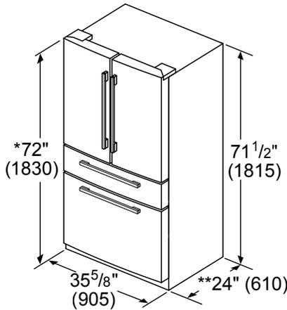
\* Add  $\frac{5}{8}$ " (17) with front leveling feet fully extended
