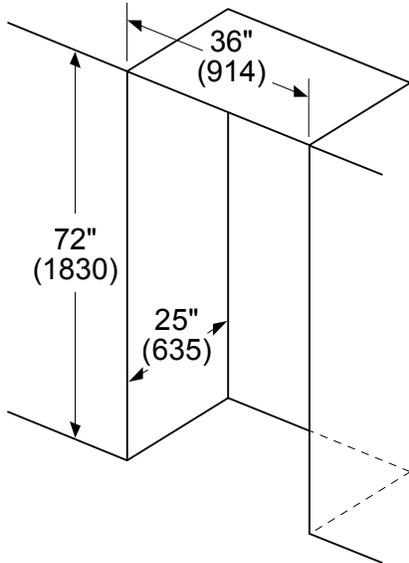
Leave 1/2" (12.7) gap at the top and 1" (25.4) behind the refrigerator for proper ventilation.
