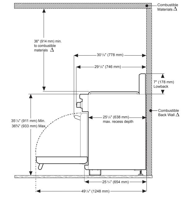
▲ As defined in the "National Fuel Gas Code" (ANSI Z223.1, Current Edition). Clearances from non-combustible materials are not part of the ANSI Z21.1 scope and are not certified by CSA. Clearances of less than 12" (305 mm) must be approved by the local codes and/or by the local authority having jurisdiction.
