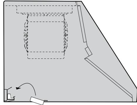
3. Start with an outside filter. Slide the filter up, toward the front of the hood, then push down on top of the grease tray.
