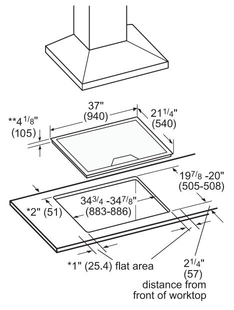
\* Minimum distance from cutout to the wall \*\* Recessed depth (includes 1" air clearance)
