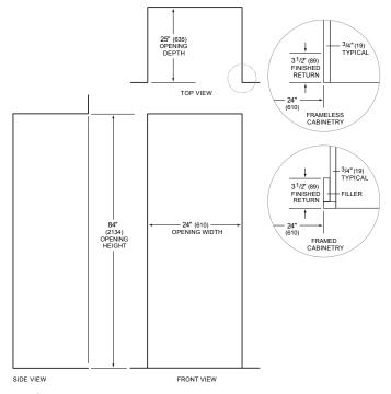
$NOTE: 3^{1}\!/2^{*}(89) \text{ finished returns will be visible and should be finished to match cabinetry}$
