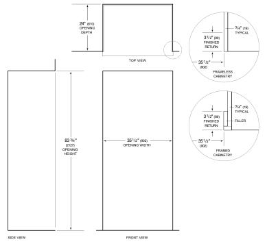
NOTE:  $3^1/2^n$  (89) finished returns will be visible and should be finished to match cabinetry Shaded line represents profile of unit.
