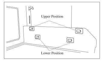
Use the correct accessories provided for each cooking mode. Place accessories in the correct installation position and direction.
