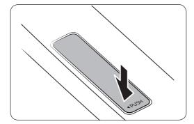
**1.** To unlock the adapter cover, press the cover to the left of the word PUSH as shown in the illustration.
