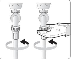
To connect the water hoses to the faucets: **1.** Connect one end of each water hose to
