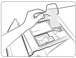
**3.** Add fabric softener to the **softener compartment**. Do not exceed the **max line** (A).
