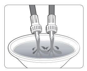
**4.** Put the other ends of the hoses into a bucket and open the taps for 10-15 seconds to remove impurities. When done, close the taps.
