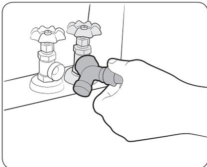
1. Close the cold water tap. If you have a washer's cold water hose attached to the cold water tap, unscrew and remove the hose. Then, connect the female end of the Y-connector to the cold water tap.
