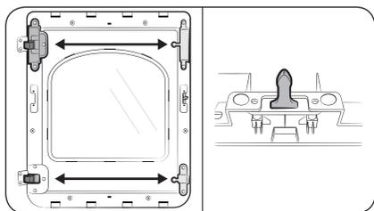
8. Remove the glass holder, and switch the positions of:
