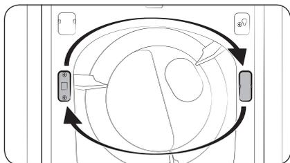
4. Remove the two screws from the lever holder, and then remove the holder cover.
