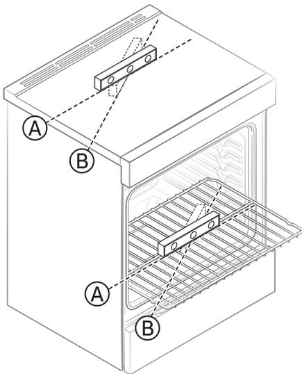
Use a spirit level to check your adjustments. Place the level diagonally on the oven rack or surface cooktop, and confirm the range is level in the two directions shown below.
