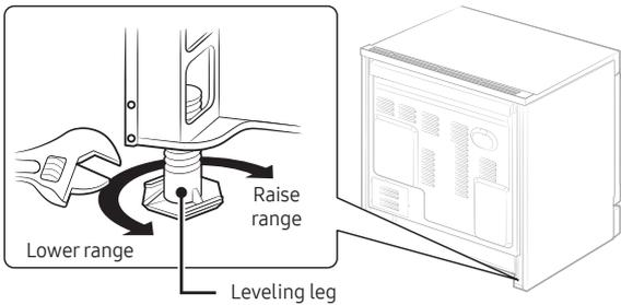
Level the range by adjusting the leveling legs with a wrench.
