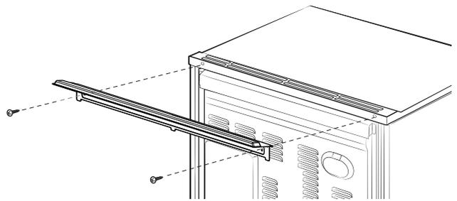
2. Assemble the filler strip to the back of the range using the removed screws.
