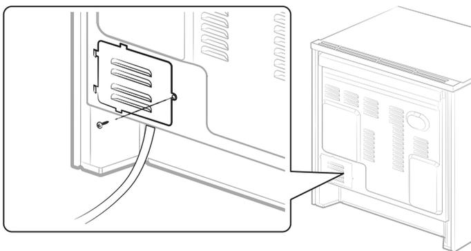
To replace the rear access cover on the range back. Insert the double projections on the bottom of the cover into the pockets located below the opening, and then insert and tighten the rear access cover screw.
