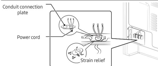
For power cord installations, hook the strain relief over the power cord hole (1 $\frac{3}{8}$ " ) located below the rear of the drawer body. Insert the power cord through the strain relief and tighten the device.
