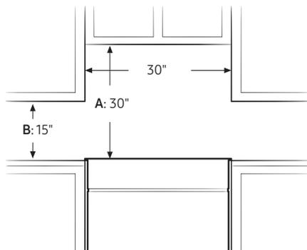
**IMPORTANT:** To eliminate the risk of burns or fire caused by reaching over heated surface units, avoid having cabinet storage space located above the surface units. If you have cabinet storage space over the heating elements, you can reduce the risk by installing a range hood that projects horizontally a minimum of 5 inches beyond the bottom of the cabinets.
