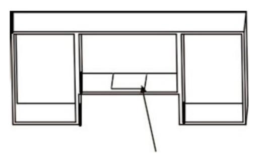
• Use the diagram below for correct placement of ductwork and electrical cut-out in cabinets.
