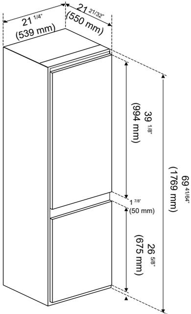
**Installation before using the appliance** Make sure there is enough space around the refrigerator to allow it work properly. A free space of 1cm (1/4inch) is required on the rear of the appliance so that the air can be circulated to cool the compressor and condenser. And 30cm (12inches) space above the refrigerator.
