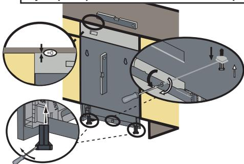
If the height of the enclosure is above 35 7/8" (910mm) use long supports as shown in the figure.
