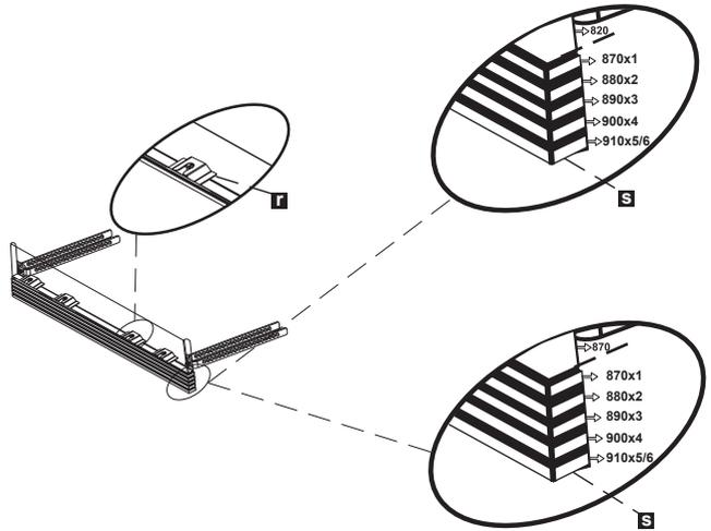
3. Depending on the desired depth, plinth locking (y) is attached to the toe kick bracket (o).
