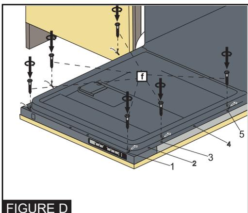
7- As shown in Figure D, Screws  $\text{Ø } 5/32'' \times 53/32''$  ( $\text{Ø } 4\text{mm} \times 42,5\text{mm}$ ) is installed in positions I, III and V.
