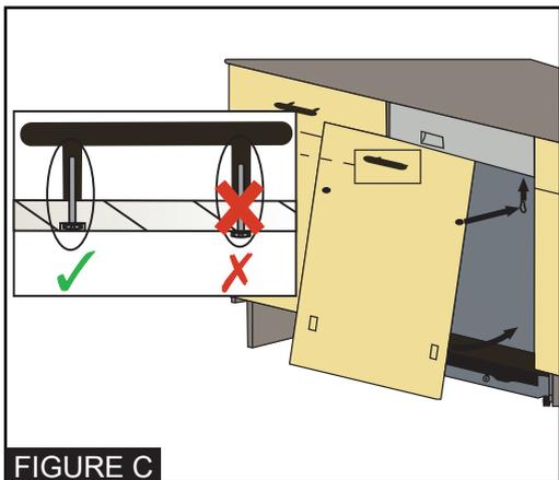
5- Before mounting the wooden door on the dishwasher, mount the handle on the wooden door as in figure C.
