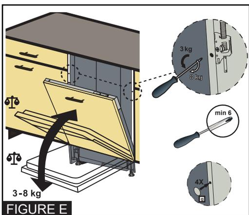
8- According to the weight of the assembled wooden door, the balancing must be provided by the mechanism shown in Figure E.
