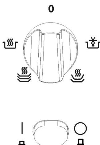
The control panel has a function and the on/off switch. The control panel is only visible when the drawer is open.
