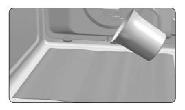
2. Gently pour 200 ml of water into the bottom of the oven cavity.
