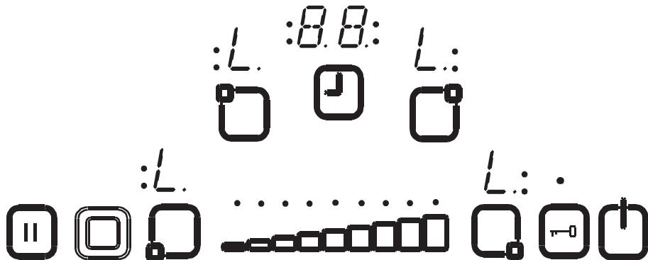
If case the minute minder is still running, it will proceed until '00' is reached and the timer will beep. After confirmation of timer run out, the appliance is fully locked. None of the buttons can be used as long as the appliance is locked.
