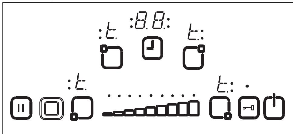
After cooktop temperature falls, the 't' displays will be erased and the cooktop control unit falls back into the S-Mode. This means that the user can reactivate the appliance by touching .
