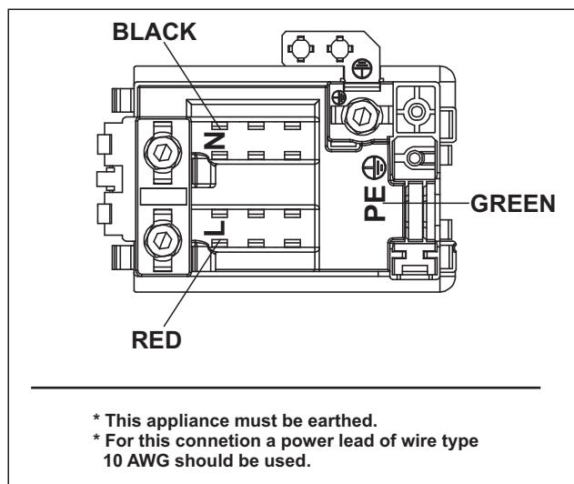
For the induction cooktop, the cable must be suitable for region will be used. You will find the connection diagram shown on the bottom of your appliance.
