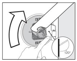
■ Open the cover and use the wrench supplied with the washing machine to turn the shipping strut 90°.
