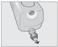
Remove the cover cap from the cartridge.
