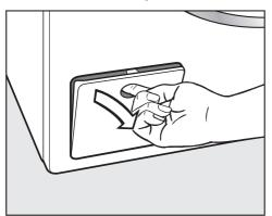
Open the drain pump flap.
