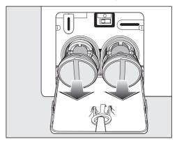
■ Remove the drain filters completely.
