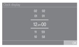
Enter the numbers by swiping upward or downward. Place your finger on the number that you want to change and move your finger in the direction you want. Touch the OK sensor button to accept the set numerical value.
