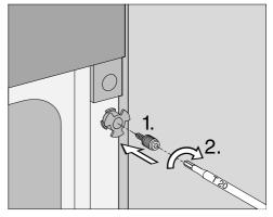
■ Insert the bolt into the mounting aid and tighten it in the cabinet niche.
