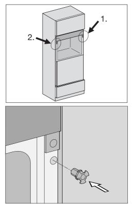
Insert the mounting aid into the hole in the front frame.
