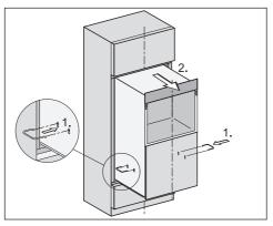
Pull the oven out of the housing unit until the holes for the carry handles are visible (1.).
