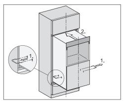
Remove the carry handles (1.). Keep the carry handles in case the oven needs to be moved again in the future. Push the oven all the way into the housing unit and align it in the center of the unit (2.).
