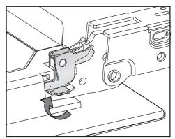
To relock the locking clamps, turn them back up to the horizontal position as far as they will go. With the help of the following guide minor faults in the performance of the machine, some of which may result from incorrect operation, can be remedied without contacting the Service Department. Time and money will be saved because a service call will not be needed.
