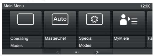
The top line shows you where you are in a menu. If you are in a submenu, you can return to the previous menu level by tapping on the desired menu name or on the boxes. The time of day, alarm, and timer appear in the top right-hand corner of the display.
