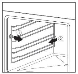
■ Pull the side runners out first at the side ①, then at the back ② of the steam oven
