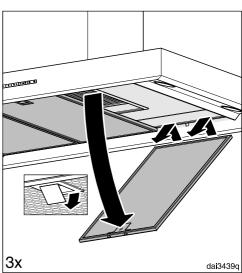
Remove the grease filters from the hood.
