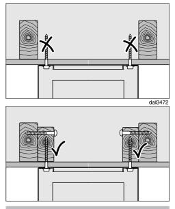
The hood must be attached to rigid structural framing that is supported in its entirety by the ceiling joists, or to the ceiling joists directly. Do not attach the plate directly to the ceiling with anchors, toggle bolts, etc.
