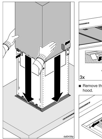
Hold the chimney securely, bend back the retaining tabs and carefully lower it.
