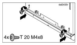
Secure the hood with the screws supplied.
