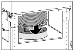
Slide the vent duct onto the vent socket and secure it (using a hose clip, for example).
