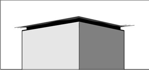
The **spacer frame** can be installed between the chimney and the ceiling. This creates a shadow which gives the illusion of a gap between the ceiling and the chimney. This is useful if the ceiling is not level or is uneven. The hood is aligned vertically with the spacers supplied. Visual irregularities between the chimney and the ceiling are then concealed by the shadow.
