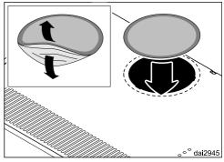
■ For operation in the recirculation mode, attach the cover foil to the opening at the back of the range hood. The foil comes with the OdorFree Charcoal Filter (optional accessory).
