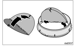
Insert the non-return flap, if required. Make sure the flap opens easily and closes again by itself.
