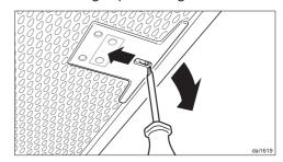
If the filters have been installed incorrectly, you can insert a small screwdriver into the slit to disengage the locking clip.
