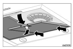
■ To remove a grease filter, release the locking clip. Then, open the filter to a 45° angle, unhook it, and remove it from the hood.
