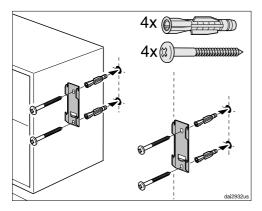
Attach the mounting brackets to the wall, using the wall anchors and screws provided.
