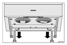
Remove the guide plugs from the housing.
