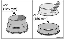
■ When using Ø 6" (150 mm) exhaust ducting, use a sharp knife to cut the exhaust socket to size with. When using Ø 5" (125 mm) exhaust ducting, install the exhaust socket as is.
