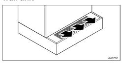
When selecting the installation position, ensure that the recirculation grille at the front of the appliance are not covered by the wall unit.
