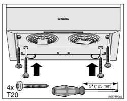
Insert the wood screws (provided) into the guide plugs and attach the hood to the cabinet floor.
