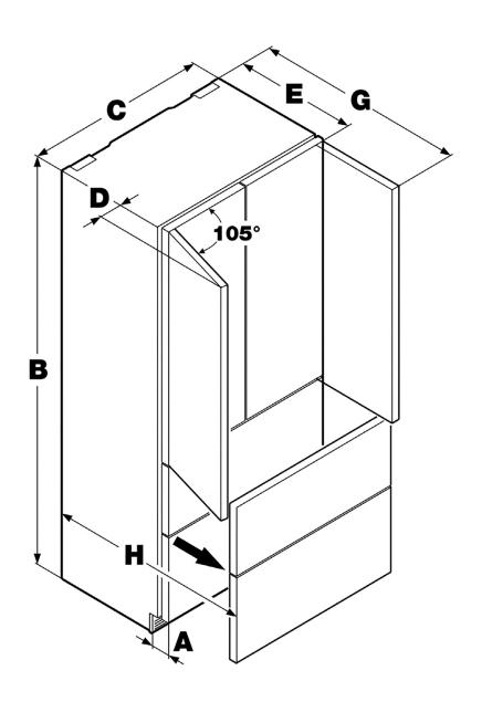
A = 3" (76 mm) B = 79-13/16" (2027 mm) C = 35-13/16" (910 mm) D = 3" (76 mm) E = 24" (610 mm) G = 42-7/16" (1078 mm) H = 37-1/8" (943 mm)
