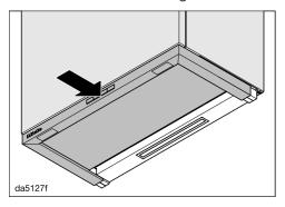
■ Carefully push in the deflector plate as far as the required position.
