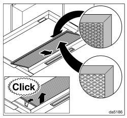
Reinsert the grease filter.
