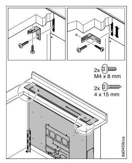
■ Fit the upper brackets loosely to the downdraft casing.
