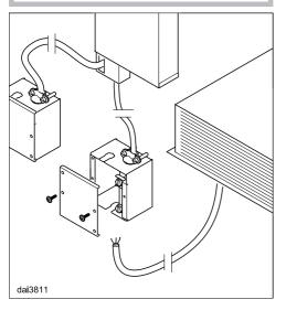
Install a connection cord from the downdraft to the external blower.
