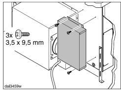
■ Fasten the connection box at a suitable location, e.g. a cabinet wall. With a DA 6891 it can be mounted on the downdraft at the indicated position to the left or right of the blower or on the back.
