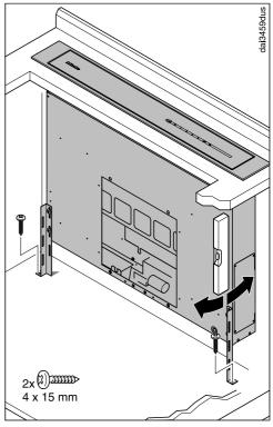
Align the downdraft vertically and screw the brackets securely to the base of the housing unit.
