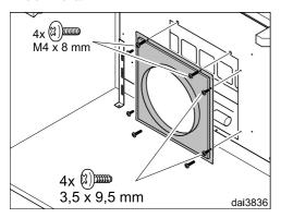
■ If an external blower is being used, the appropriate vent connector is fitted instead.
