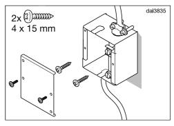
■ Secure the connection box to a suitable place, e.g. a cabinet wall.
