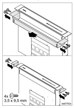
Unscrew the screws on either side, remove the support bracket and replace it with the two small angle brackets supplied.
