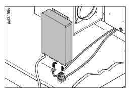
Guide the two connection cords on the bottom of the downdraft through the casing and plug them into the appropriate sockets at the bottom of the connection box.
