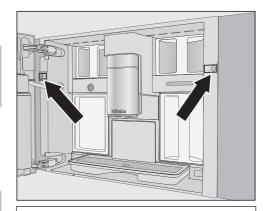
Two TX20 (25 mm) screws are included with the machine.
