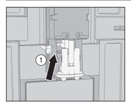
■ Detach the milk pipework from the dispensing unit as follows: pull the tab ① to the left.
