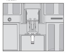
Insert the dispensing unit into the coffee machine and connect the milk pipework.
