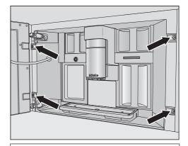
Four TX20 (25 mm) screws are supplied with the machine.
