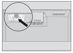
Clean the milk container holder on the coffee machine with a damp cloth.
