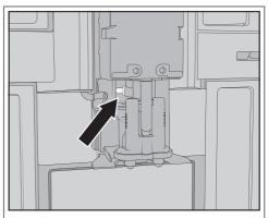
Do not remove the milk pipework connecting piece. If necessary, clean the connecting piece with the cleaning brush.
