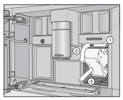
Pull the brew unit to the side ① first and then pull out to the front ②. Tilt the brew unit forward ③ while doing so.
