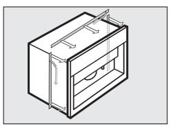
■ If there is not a seal at the front of the building-in niche, adhere the Miele sealing strips from the back (see picture) before installing the coffee system. The sealing strips can be purchased from Miele.
