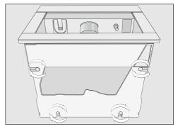
■ Using the large allen key, unscrew all four feet out by about 1/16" (2 mm).
