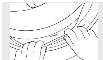
3. When you are finished cleaning the door gasket, remove your hands and the gasket will return to the operating position.
