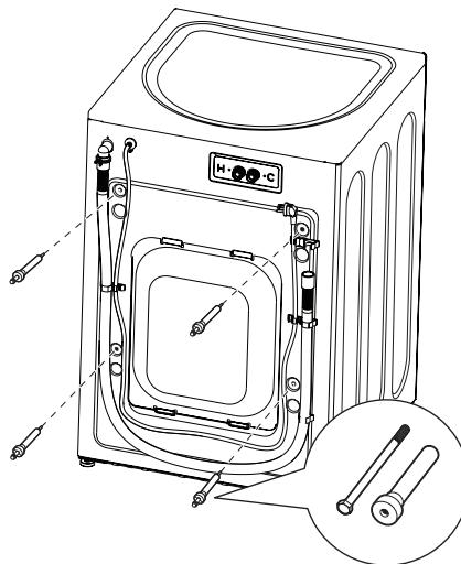
**IMPORTANT:** Failure to remove the shipping bolts\* can cause the washer to become severely unbalanced.
