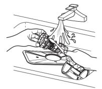
5. Reassemble the filters in the reverse order of the disassembly, replace the filter insert, and rotate clockwise to the close arrow.
