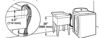
Minimum capacity: 20 gal. (76 L). Top of laundry tub must be at least 39" (990 mm) above oor; install no higher than 96" (2.44 m) from bottom of washer.
