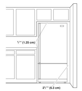
To ensure proper ventilation for your refrigerator, allow for a 1/" (1.25 cm) space on each side and at the top. Allow at least 1" (2.54 cm) between back of cabinet and the wall. If your refrigerator has an ice maker, make sure you leave some extra space at the back for the water line connections.
