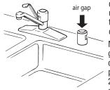
drain hose either be looped up and securely fastened to the underside of the counter or be connected to an air gap. Make sure to use an air
