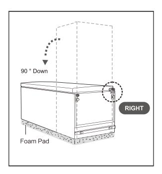
3. Remove the top hinge cover using a flat head screwdriver and then remove the screws using a Philips screwdriver. Move the top hinge to the opposite side and re-attach it to the cabinet.
