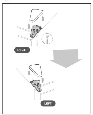
2. Then unload the down hinge, the support plate and the door limit block and fix to the left side with adjustable wrench and a cross screwdriver, as shown in the picture
